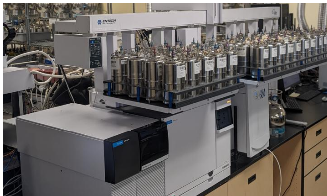
Fig 5. Automated GC-MS/MS instrumentation for OTM-50
