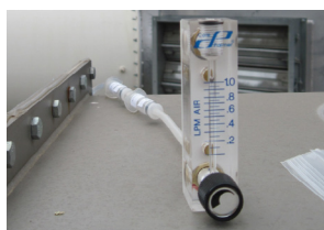
Figure C. Flow is marked by small metal ball. To decrease flow, turn black dial clockwise.
