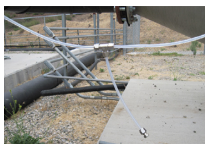
Figure A. One side should attach to gas outlet while the other attaches to calibration tubes.
