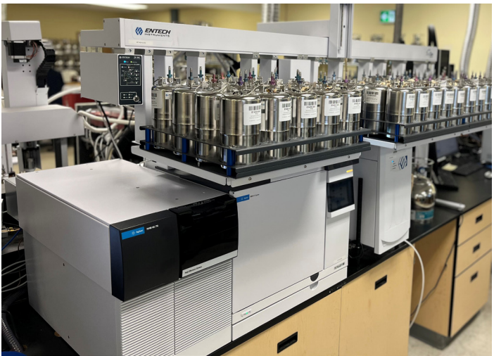
Fig 5. Automated GC-MS/MS instrumentation for OTM-50
