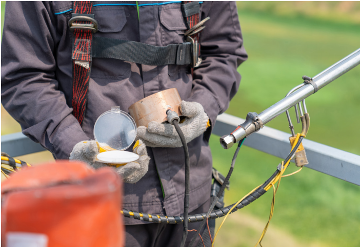
Fig 4. Field sampler assembling sampling probe and inlet filter for OTM-50 canister sampling
