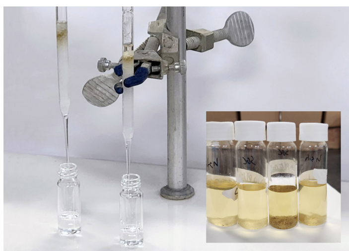
Fig 3. Silica gel column cleanup (left); in-situ cleanup (inset)
