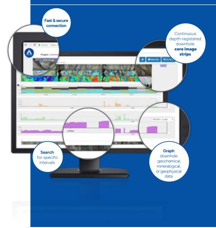
Using core photos taken by ALS or provided by you over a secure connection, we create continuous depth-registered downhole core image strips. The box photos and core strips are available to you through CoreViewer™, where you can search for specific intervals and graph any kind of downhole geochemical, mineralogical, or geophysical data for comparison against the images.
