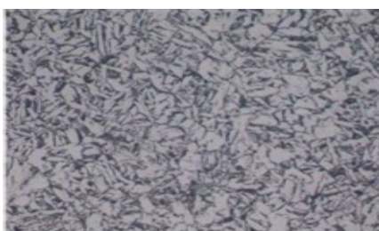
Microstructure of the bulk material of the component
