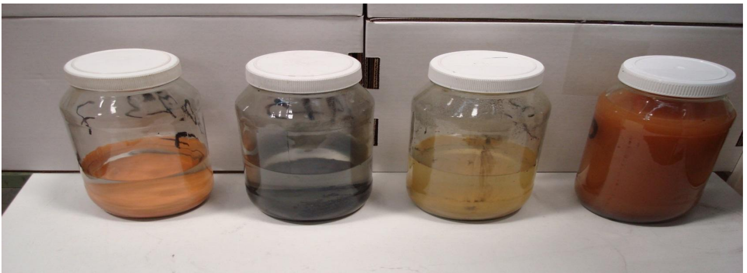
Plate 2. TCLP jars containing leached solids and leachate solutions
