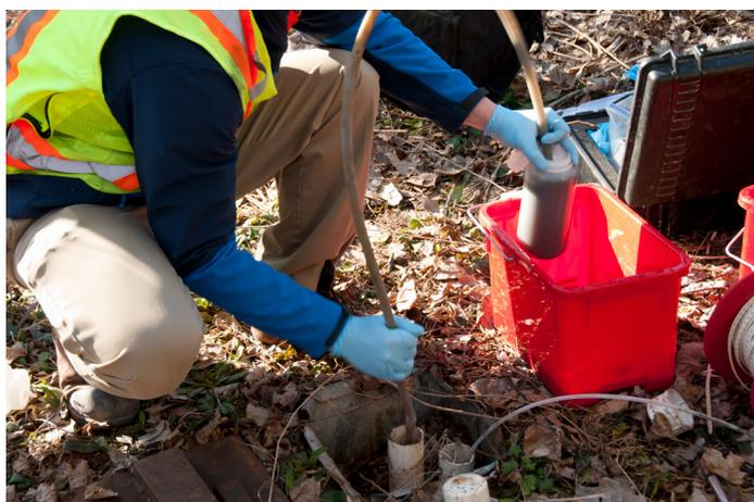
Figure 3. Collection of disturbed groundwater sample
