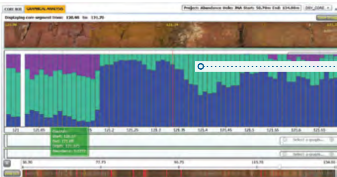
Example data integration using HyLogger™ continuous scanning in combination with core images.
