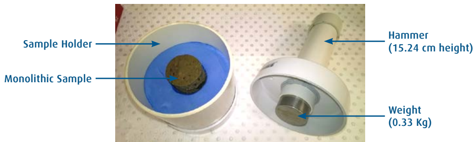
Figure 2. Opened Structural Integrity Tester with monolithic sample in position
