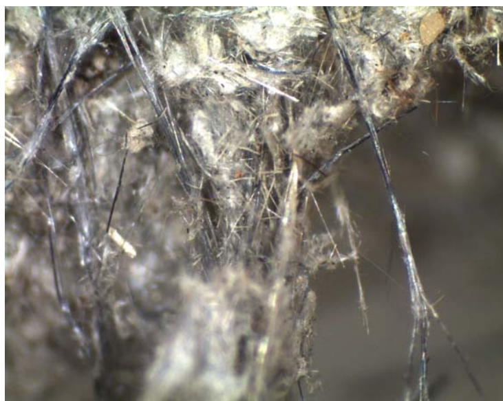
Mixed Asbestos Insulation At 28x Magnification
